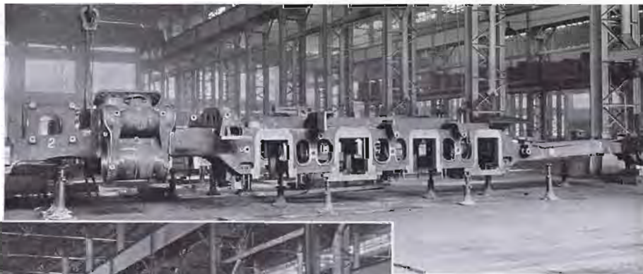
One-Piece, Cast-Steel Locomotive Bed With Cylinders, Back Cylinder Heads, Air Reservoirs, and Other Parts Cast Integral.
