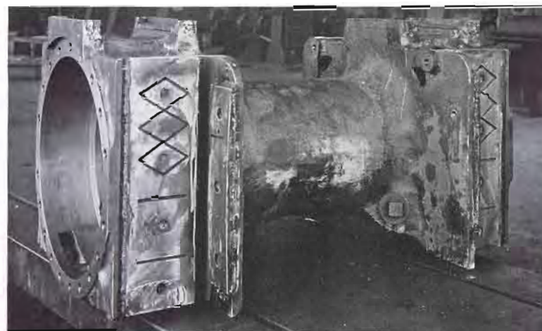
One-Piece Housing of the Timken Roller Bearings Applied to the Driving Axles.
