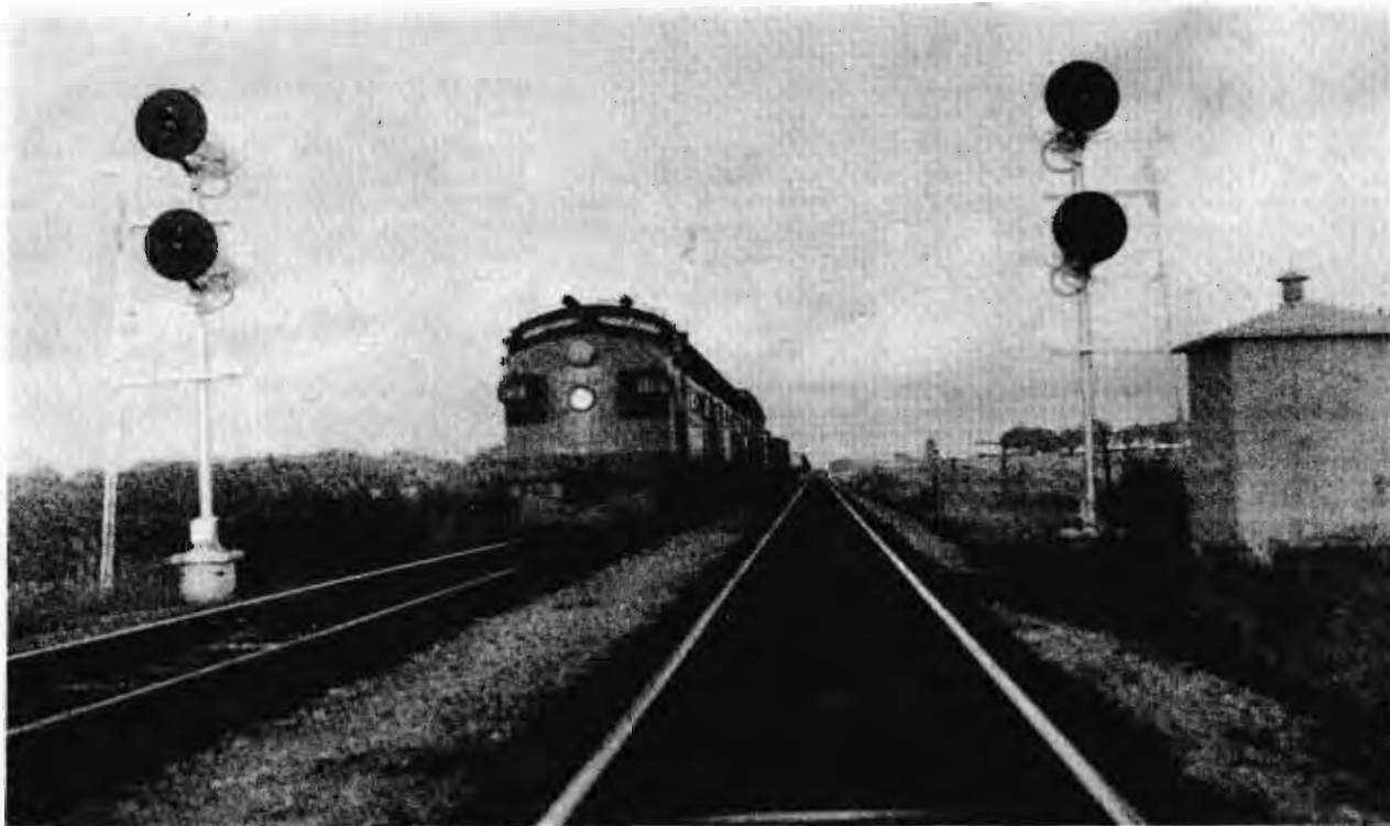
TRAIN MOVEMENTS signaled both ways on each track of double track helped give the Milwaukee the flexibility and . . .
