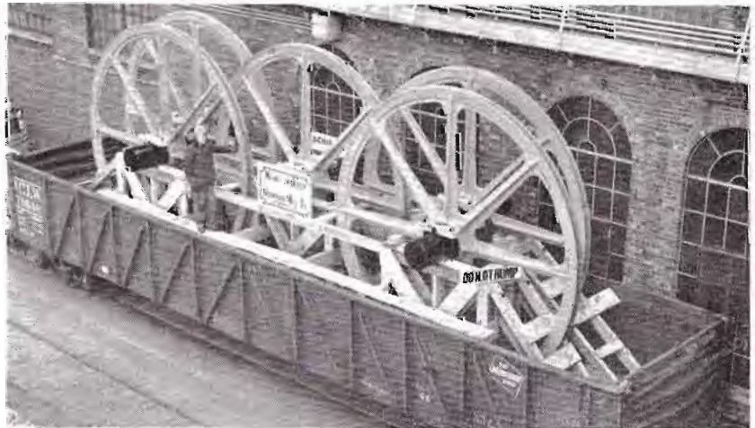
THE BIGGER THEY COME, the harder it is to stump the railroads, which continue to be the only type of transportation equipped to handle dimension loads. One which moved over The Milwaukee Road recently was this set of sheave wheels for a mine hoist, shipped by the Nordberg Mfg Co. of Milwaukee to Anaconda at Rocker, Mont. Maximum height of the shipment was 19 feet 4 inches, maximum width 10 feet. Note how the Nordberg shop man is dwarfed by its proportions.
