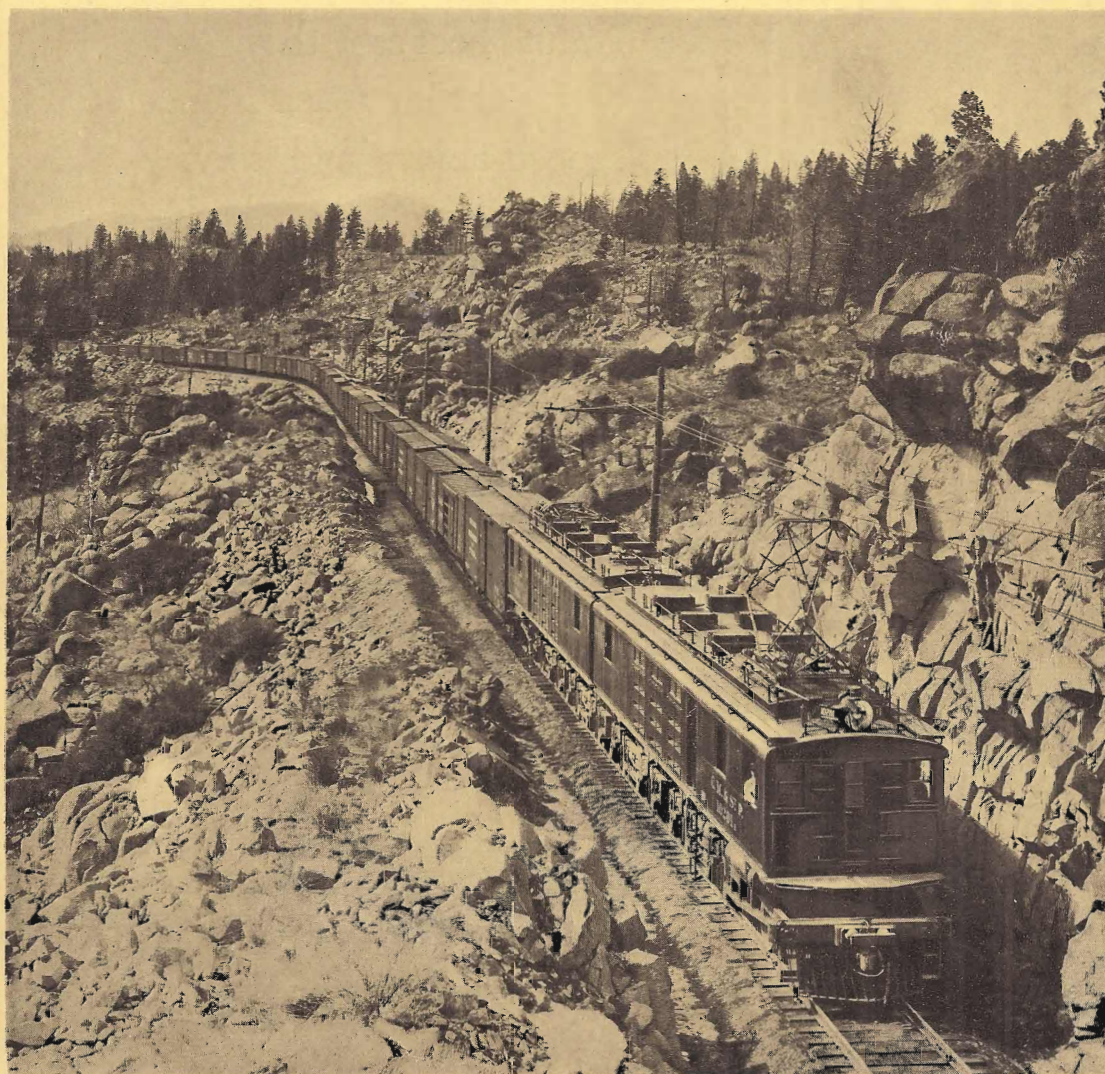
3000-VOLT DIRECT-CURRENT FREIGHT LOCOMOTIVE IN MAIN LINE SERVICE ON THE CHICAGO, MILWAUKEE & ST. PAUL RAILWAY
