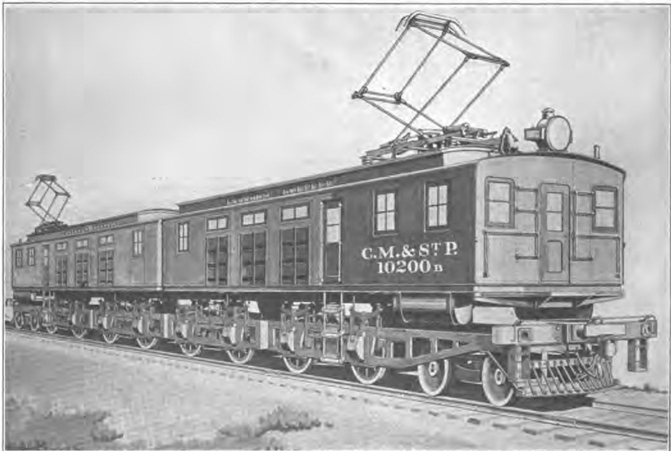
C., M. & ST. P. LOCOMOTIVE—VIEW OF COMPLETE UNIT OF WHICH TWENTY-ONE ARE NOW UNDER CONSTRUCTION. EACH LOCOMOTIVE HAS EIGHT MOTORS, TOTALING 3440 HP.
