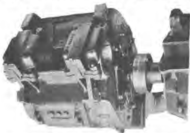
C., M. & ST. P. LOCOMOTIVE—END VIEW OF MOTOR ARRANGED FOR STAND TEST
