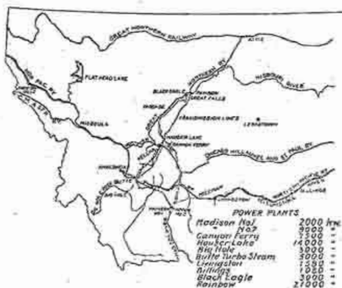
FIG. 7.—PLANTS FROM WHICH ELECTRIC POWER IS PURCHASED BY THE BUTTE, ANACONDA AND PACIFIC RAILWAY.
