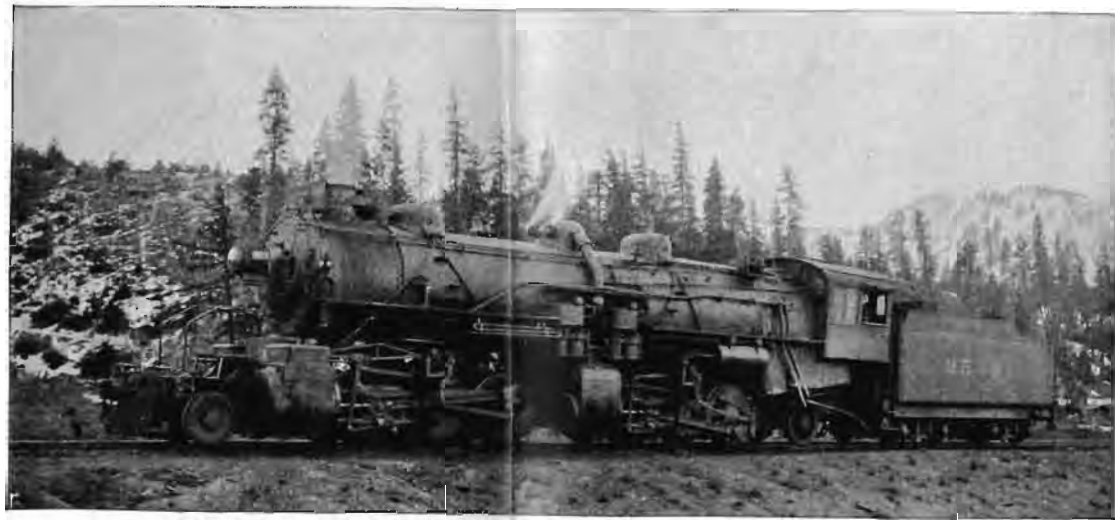
TYPE OF OIL-BURNING MALLET LOCOMOTIVE FORMERLY USED ON THE WESTERN DIVISIONS
