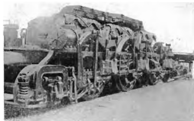
THREE TWIN MOTORS ASSEMBLED ON TRUCK
