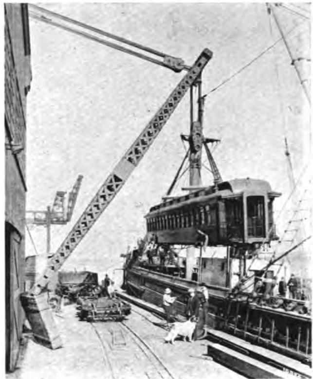
Smith's Cove terminal. The 100-ton shear leg derrick loading passenger coaches for Federal Railway in Alaska.
