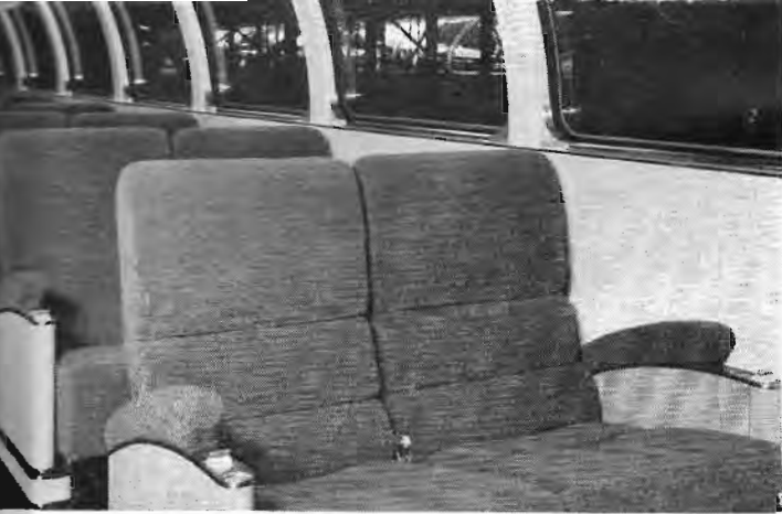
The Heywood-Wakefield seats in the full-length dome section are rubber cushioned and non-revolving.
