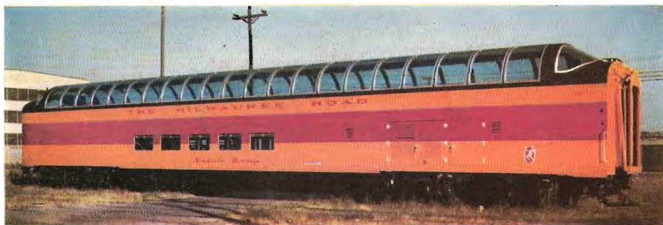
One of the Milwaukee "Super-Dome" cars with curved double-glazed high-visibility windows in the full-length dome.
