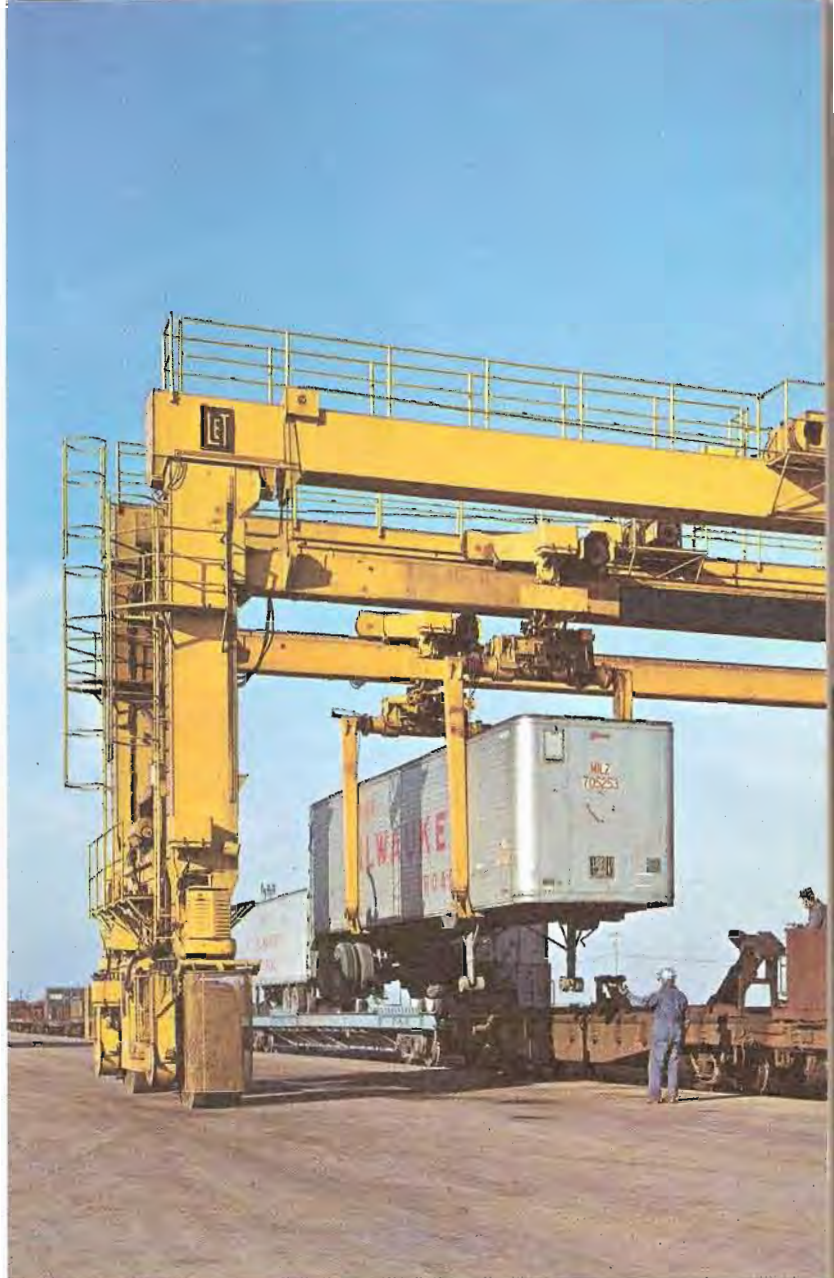
● Giant gantry crane lifts trailer onto flat car at Bensenville Piggyback Park.
