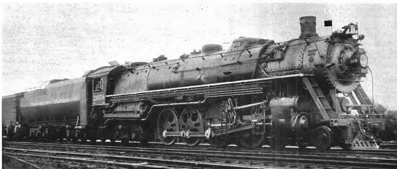
One of the Ten 4-8-4 Type Locomotives Built by Baldwin for the Northern Pacific in 1934.
