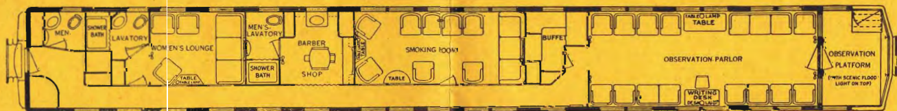
The All-luxury Observation Car. Barber Shop—Baths for Men and Women—Women's Lounge—Smoke Room—Buffet—Library—Observation Parlor
