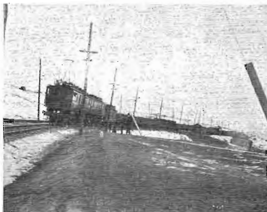
Figs. 5 and 6. Exhibition Test of Chicago, Milwaukee and St. Paul Locomotives on 1.66 per cent Grade near Janney Substation. Three steam locomotives operating at 9-10 m.p.h. with 2000 tons trailing; two electric locomotives operating at 15-16 m.p.h. with 3000 tons trailing
