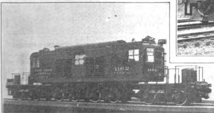
One of the latest types of gearless-drive locomotives, which have been found very satisfactory during the past ten years by the New York Central Railroad on its New York-Harmon division.
