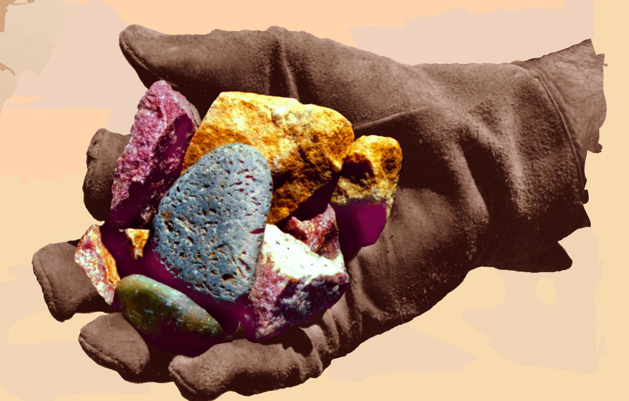
he rails and ties on this part from passing trains, allowed of the line sat on a rock bed of water to drain and protected distinctive, colorful quartzite ballast mined from quarries 85 miles away in Montana.
