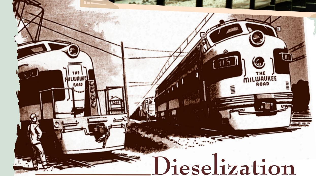
Glamourous and dependable steam locomotives couldn't match the efficiency of diesel locomotives. Diesels saved 70 to 80 percent on fuel costs over oil or coal fired steam engines, required less maintenance and needed fewer men to operate.
