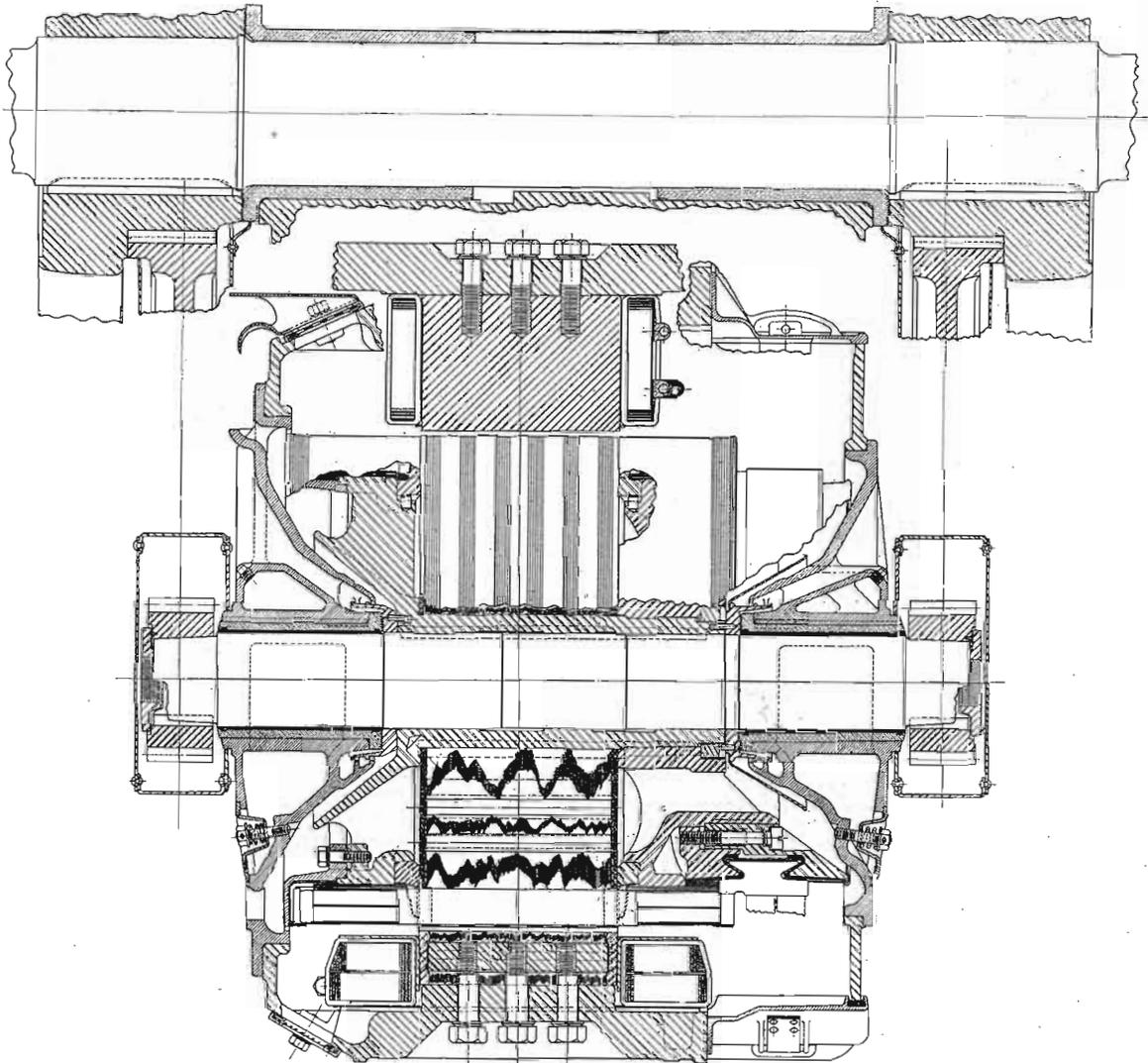
Fig. 3. Longitudinal Section of Motor
