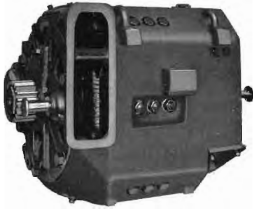
GE-229 1200 VOLT MOTOR SHOWING OPENING FOR VENTILATING PIPE
