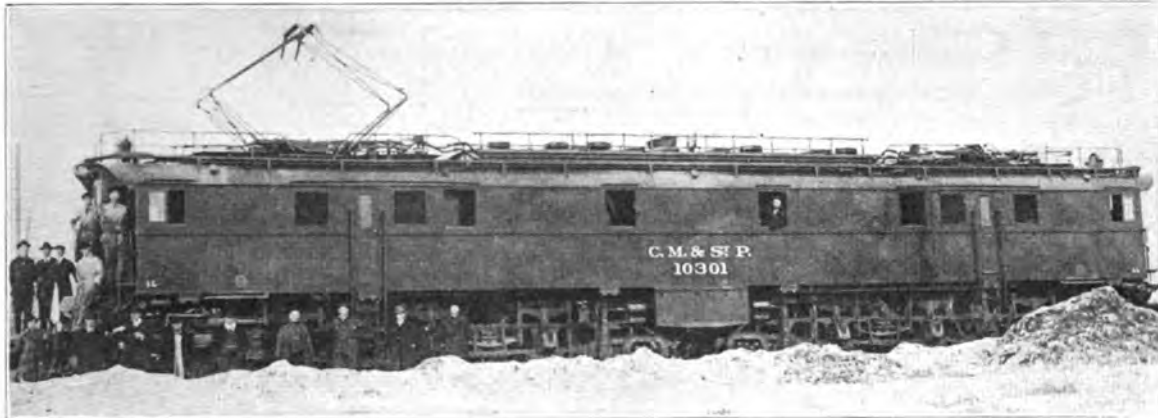
Two Hundred and Seventy-Five Ton, Twin Motor, Quill Drive, Passenger Locomotive for C. M. & St. P. Ry.
