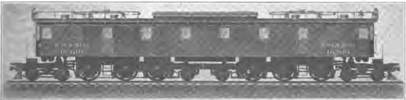
One of the Baldwin-Westinghouse 240-Ton Electric Passenger Locomotives for the Chicago, Milwaukee & St. Paul Railway.
