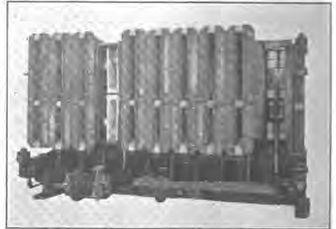
Series-Parallel Switch Group. These Switches are Air Operated
