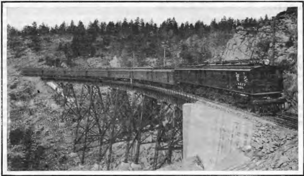
SINGLE ELECTRIC UNIT HANDLES SEVEN AND EIGHT COACHES ON 2-PER CENT GRADES
