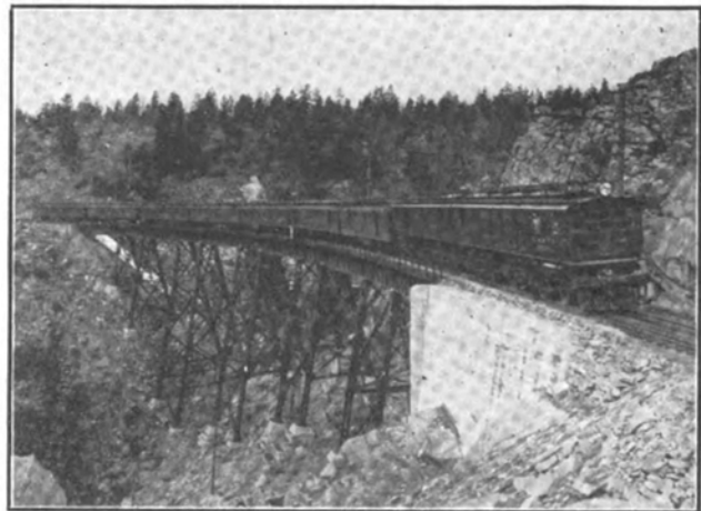
Chicago, Milwaukee & St. Paul Electrified Freight and Passenger Trains, Descending Two-Per-Cent Grade on Eastern Slope of Rocky Mountains. Double-Unit, 3,000-Volt, Direct-Current Locomotives Used.
