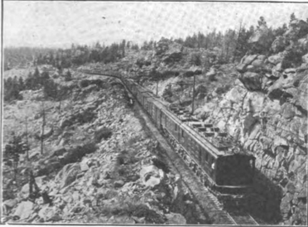
Chicago, Milwaukee & St. Paul Electrified Freight and Passenger Trains, Descending Two-Per-Cent Grade on Eastern Slope of Rocky Mountains. Double-Unit, 3,000-Volt, Direct-Current Locomotives Used.
