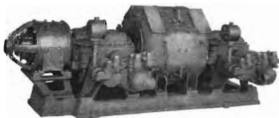
Fig. 16. 3000-volt Compressor Exhaust Set Geared to Control Generator
