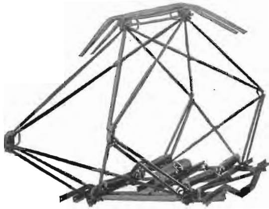
Fig. 2. 3000-volt Pantagraph Trolley Shown in Raised Position
