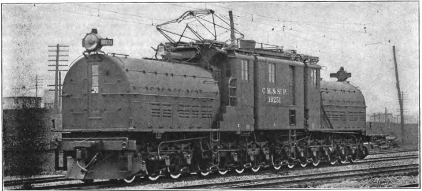
NEW 3000-VOLT DIRECT-CURRENT GEARLESS PASSENGER LOCOMOTIVE, WEIGHING 265 TONS, FOR THE ST. PAUL CASCADE ELECTRIFICATION
