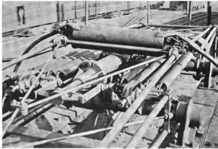
Fig. 19. A Pantograph Folded showing Revised Wear Plate
